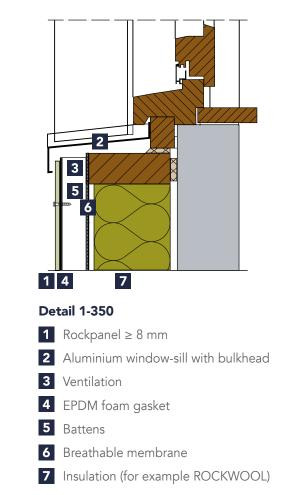
Mechanically fixed to timber supports, junction at window head
